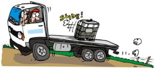
Unrestrained IBCs will move in transit and must be restrained with fit for purpose load restraint devices.
