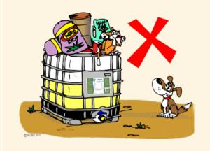
Storing chemical drums and other products on IBCs may damage the IBC and potentially contaminate the IBC.
