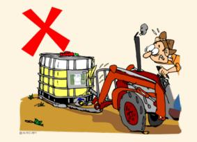
Often on farms the only practical option for lifting IBCs involves the use of tractors with hydraulic lifting devices. Hay forks should not be used as they are often bent and can be slippery.
