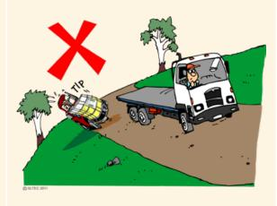
Forklifts are not all terrain vehicles and they must only ever be operated on flat terrain with compacted gravel hard strand traffic surfaces.
